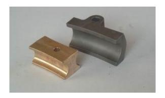
The counterformer is used to bend thin pipes. The diameter of the pipe in mm/inches/ gas inches is written on the counterformer.
