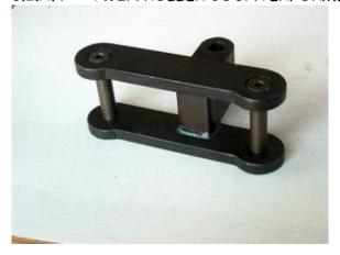
The counterformer for the twin rollers is used to bend pipes whose thickness exceeds 2,5 mm (it is used with two rollers on the basis of the pipe to bend); the use of this tool avoids the pipe flattening.
