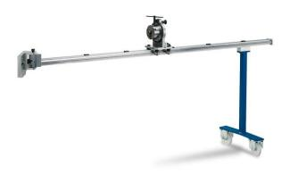
Moving arm equipped with an angle of plane regulator to make sequential bends on the same pipe on different plans. Available from 1 - 2 - 3 - 4 metres.
