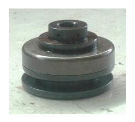
Three universal rollers for ring rolling structural sections and plates (the picture shows one single universal roller).
