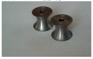
They are to be used with the twin roller counterformer.
